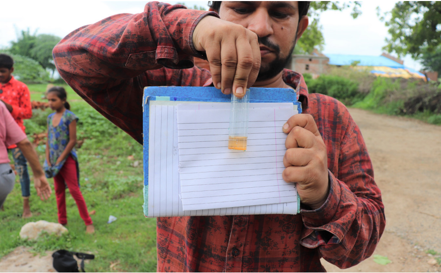
The INREM team visits wells and lakes around the village of Fatepura and tests the water using a test tube filled with a reactive agent
